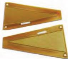
triangular MFC for strain adaptation
