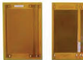
sensor/actuator arrays for closed loop control
